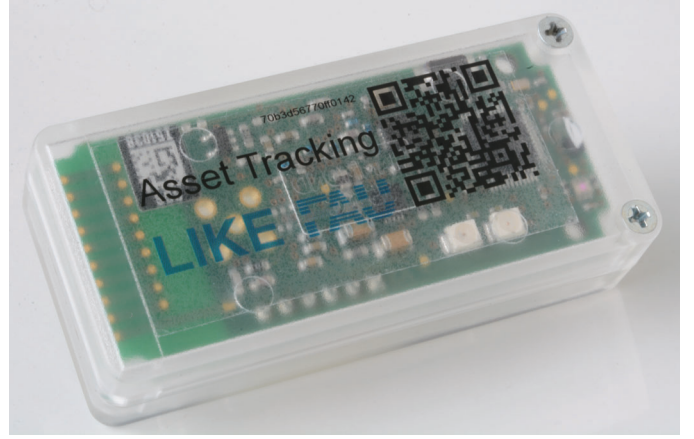
Fig. 8. Image of the sensor node used in the measurements. The size of the complete sensor node is approx. 60 \times 30 \times 15 mm.
