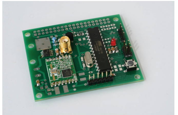
Fig. 9. LPWAN sensor node for calibration purposes.
